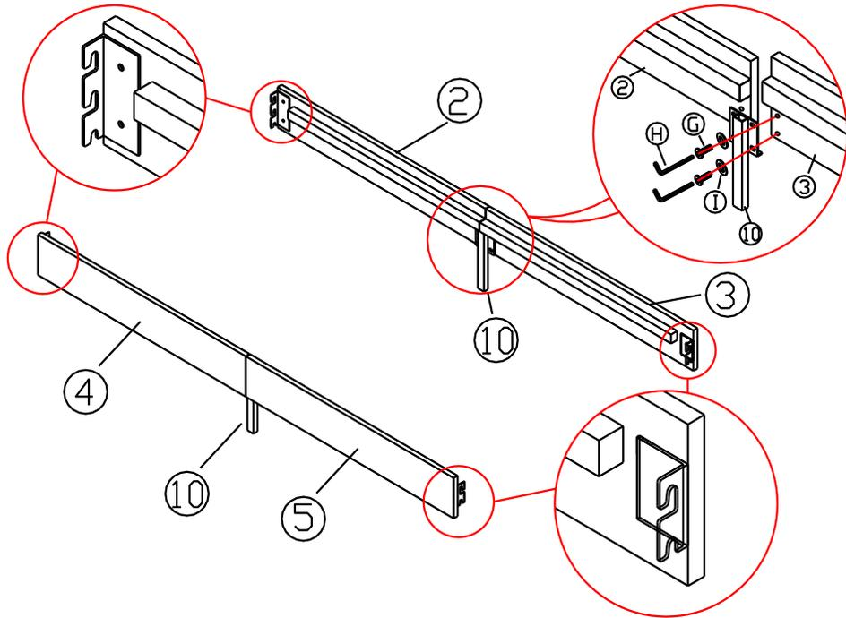
Attention: Please align the two rails tightly before tightening the bolts.
